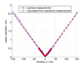
Figure 3: Comparison of the beam diameter measured with the camera and calculated from the wave-front measurement.
