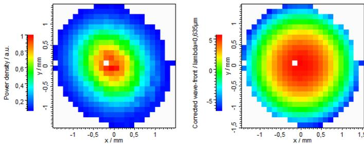
Figure 2: Intensity distribution and wave-front measured with SHSLab in the divergent part of the beam.
