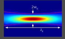
Single shot measurement of phase and intensity: Calculation of beam waist radius  $W_0$ , Rayleigh range  $Z_g$ , beam waist position  $Z_0$  and  $M^2$ .
